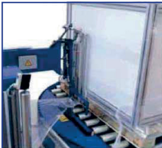
Cutting Unit: Binding film and cutting automatically.
